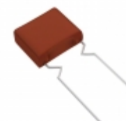
ECW-F2154HAQ Panasonic Electronic Components CAP FILM 0.15UF 3% 250VDC RADIAL
