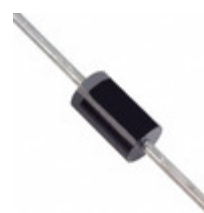
1N5820-B Diodes Incorporated DIODE SCHOTTKY 20V 3A DO201AD
