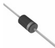
1N5820 B0G TSC (Taiwan Semiconductor) DIODE SCHOTTKY 20V 3A DO201AD
