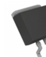
BA78M08FP-E2 Rohm Semiconductor IC REG LDO 8V 0.5A TO252-3
