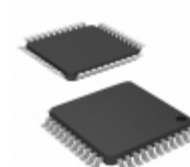
DSPIC30F4011-30I/PT Microchip Technology IC MCU 16BIT 48KB FLASH 44TQFP
