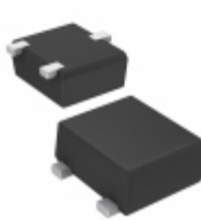
2SD2701TL Rohm Semiconductor TRANS NPN 12V 2A TUMT3
