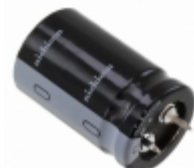
LLS2E391MELZ Nichicon CAP ALUM 390UF 20% 250V SNAP
