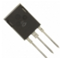
APT100GT60B2RG Microsemi Corporation IGBT 600V 148A 500W SOT247
