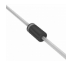
BZW04-28-E3/54 Electro-Films (EFI) / Vishay TVS DIODE 28.2V 45.7V DO204AL
