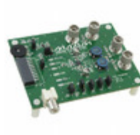
MAX9768EVKIT+ Maxim Integrated EVALUATION KIT FOR MAX9768
