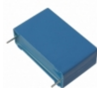
B32676G3206K EPCOS (TDK) CAP FILM 20UF 10% 300VDC RADIAL
