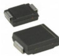
SM30T33AY STMicroelectronics TVS DIODE 28VWM 45.4VC SMC
