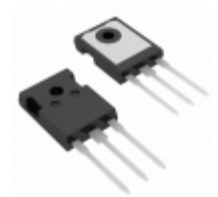
IXSH50N60B IXYS IGBT 600V 75A 250W TO247
