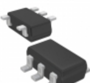
XC6122E441MR-G Torex Semiconductor Ltd IC WATCHDOG TIMER SOT-25
