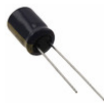
EEU-FC2A390LB Panasonic Electronic Components CAP ALUM 39UF 20% 100V RADIAL
