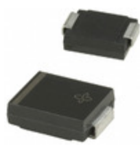
SMCJ48C-E3/9AT Vishay Semiconductor Diodes Division TVS DIODE 48VWM 85.5VC SMC
