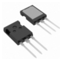
IXGX50N120C3H1 IXYS IGBT 1200V 95A 460W PLUS247
