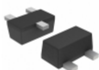
DTA023YEBTL Rohm Semiconductor TRANS PREBIAS PNP 50V 0.15W SC89
