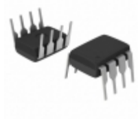
NCP1000P ON Semiconductor IC OFFLINE SWIT PWM UVLO HV 8DIP
