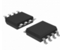
BA3404FJ-GE2 Rohm Semiconductor IC OP AMP GROUND SENSE SOP8J
