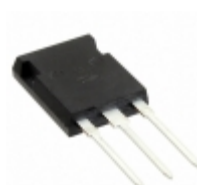
APT35GA90B Microsemi Corporation IGBT 900V 63A 290W TO-247
