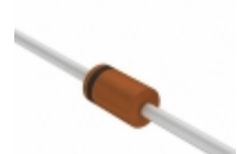
MTZJ8V2SB R0G TSC (Taiwan Semiconductor) DIODE ZENER 7.99V 500MW DO34
