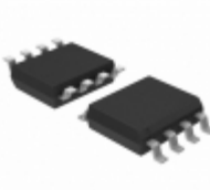
SY10EP05VZI-TR Microchip Technology IC GATE AND/NAND 3.3V/5V 8-SOIC
