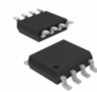
ACSL-6210-50R Avago Technologies (Broadcom Limited) OPTOISO 2.5KV 2CH OPEN COLL 8SO
