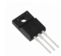
BA07CC0T Rohm Semiconductor IC REG LDO 7V 1A TO220FP
