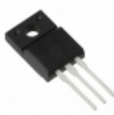
BA07T Rohm Semiconductor IC REG LDO 7V 1A TO220FP
