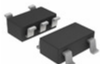
NCP4688DSN33T1G ON Semiconductor IC REG LDO 3.3V 0.15A SOT23-5
