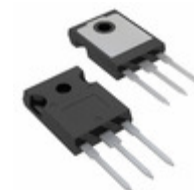
IRFP4568PBF Infineon Technologies MOSFET N-CH 150V 171A TO-247AC
