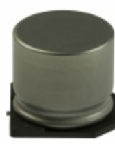
EEE-FK1J681AM Panasonic Electronic Components CAP ALUM 680UF 20% 63V SMD
