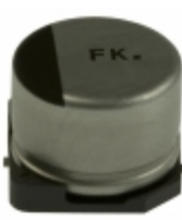
EEE-FK1J470P Panasonic Electronic Components CAP ALUM 47UF 20% 63V SMD
