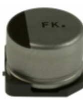
EEE-FK1K100P Panasonic Electronic Components CAP ALUM 10UF 20% 80V SMD
