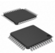
DSPIC33FJ16GS504-H/PT Micrel / Microchip Technology IC MCU 16BIT 16KB FLASH 44TQFP
