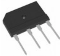
TS40P06GHD2G TSC (Taiwan Semiconductor) BRIDGE RECT 1P 800V 40A TS-6P
