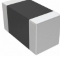
CC1206KKX7R7BB475 Yageo CAP CER 4.7UF 16V X7R 1206
