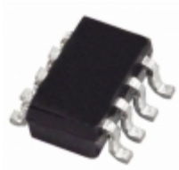
ADG3249BRJ-REEL Analog Devices Inc. IC MUX/DEMUX 2X1 SOT23-8
