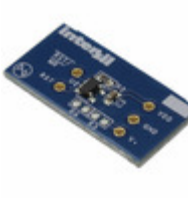
ISL88012EVAL1Z Intersil EVALUATION BOARD FOR ISL88012
