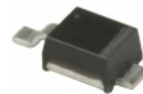
1PMT4135CE3/TR13 Microsemi Corporation DIODE ZENER 100V 1W DO216
