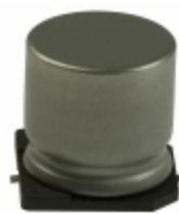
EEE-FK1A472AM Panasonic Electronic Components CAP ALUM 4700UF 20% 10V SMD
