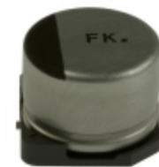
EEE-FK1A471P Panasonic Electronic Components CAP ALUM 470UF 20% 10V SMD
