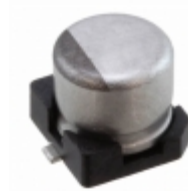
UZR1V4R7MCL1GB Nichicon CAP ALUM 4.7UF 20% 35V SMD
