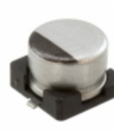
UZR1V100MCL1GB Nichicon CAP ALUM 10UF 20% 35V SMD
