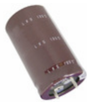
ELXS421VSN221MP50S United Chemi-Con CAP ALUM 220UF 20% 420V SNAP
