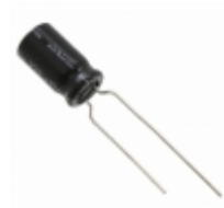
UVR2ER47MED1TA Nichicon CAP ALUM 0.47UF 20% 250V RADIAL
