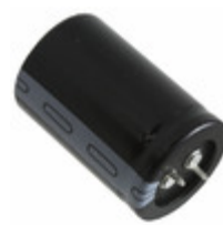
SMH63VN822M30X45T2 United Chemi-Con CAP ALUM 8200UF 20% 63V SNAP
