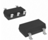
MIC5213-3.3BC5-TR Microchip Technology IC REG LDO 3.3V 80MA SC70-5
