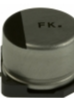
EEE-FK1C331GP Panasonic Electronic Components CAP ALUM 330UF 20% 16V SMD
