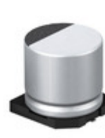
EEE-FK1C432SM Panasonic CAP ALUM 4300UF 20% 16V SMD
