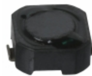
CDRH62BNP-2R9NC-B Sumida America Components Inc. FIXED IND 2.9UH 1.94A 68 MOHM
