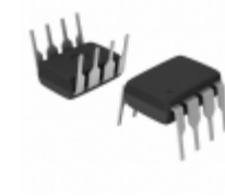
MC9S08QA4CPAE NXP USA Inc. IC MCU 8BIT 4KB FLASH 8DIP
