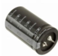
LQS2G561MELB50 Nichicon CAP ALUM 560UF 20% 400V SNAP
