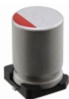
RHS0J102MCN1GS Nichicon CAP ALUM POLY 1000UF 6.3V SMD
