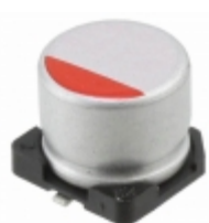
RHS0G561MCN1GS Nichicon CAP ALUM POLY 560UF 20% 4V SMD
