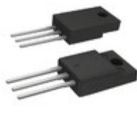
T1235T-8FP STMicroelectronics TRIAC ALTERNISTOR 800V TO220FPAB
