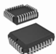
AT28HC256-70JU Microchip Technology IC EEPROM 256KBIT 70NS 32PLCC
