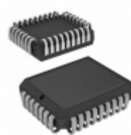
AT28C64X-25JC Microchip Technology IC EEPROM 64KBIT 250NS 32PLCC
