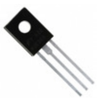
BD682S Fairchild/ON Semiconductor TRANS PNP DARL 100V 4A TO-126
