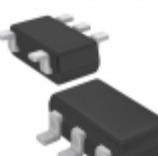
XC6123D447MR-G Torex Semiconductor Ltd IC WATCHDOG TIMER SOT-25
