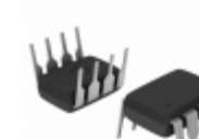
TC4424VPA Microchip Technology IC MOSFET DVR 3A DUAL HS 8DIP
